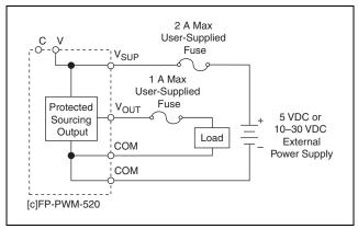
Figure 3. Wiring the [c]FP-PWM-520
